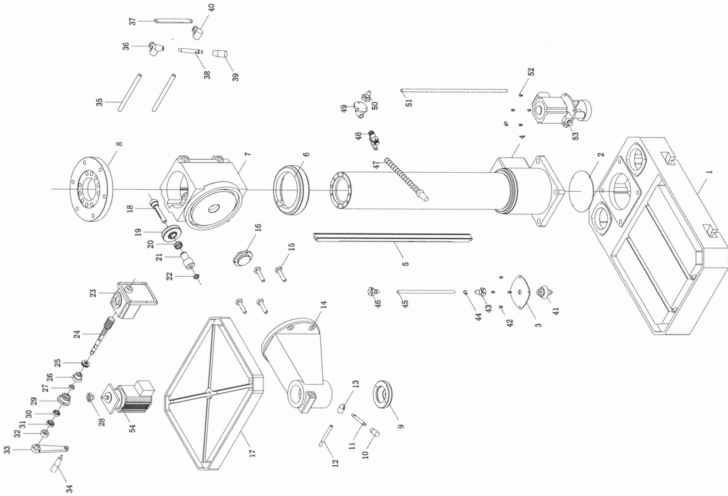
**Contrast for the parts number of GHD-55PFAL column and its bracket and its three dimension sketch.**
