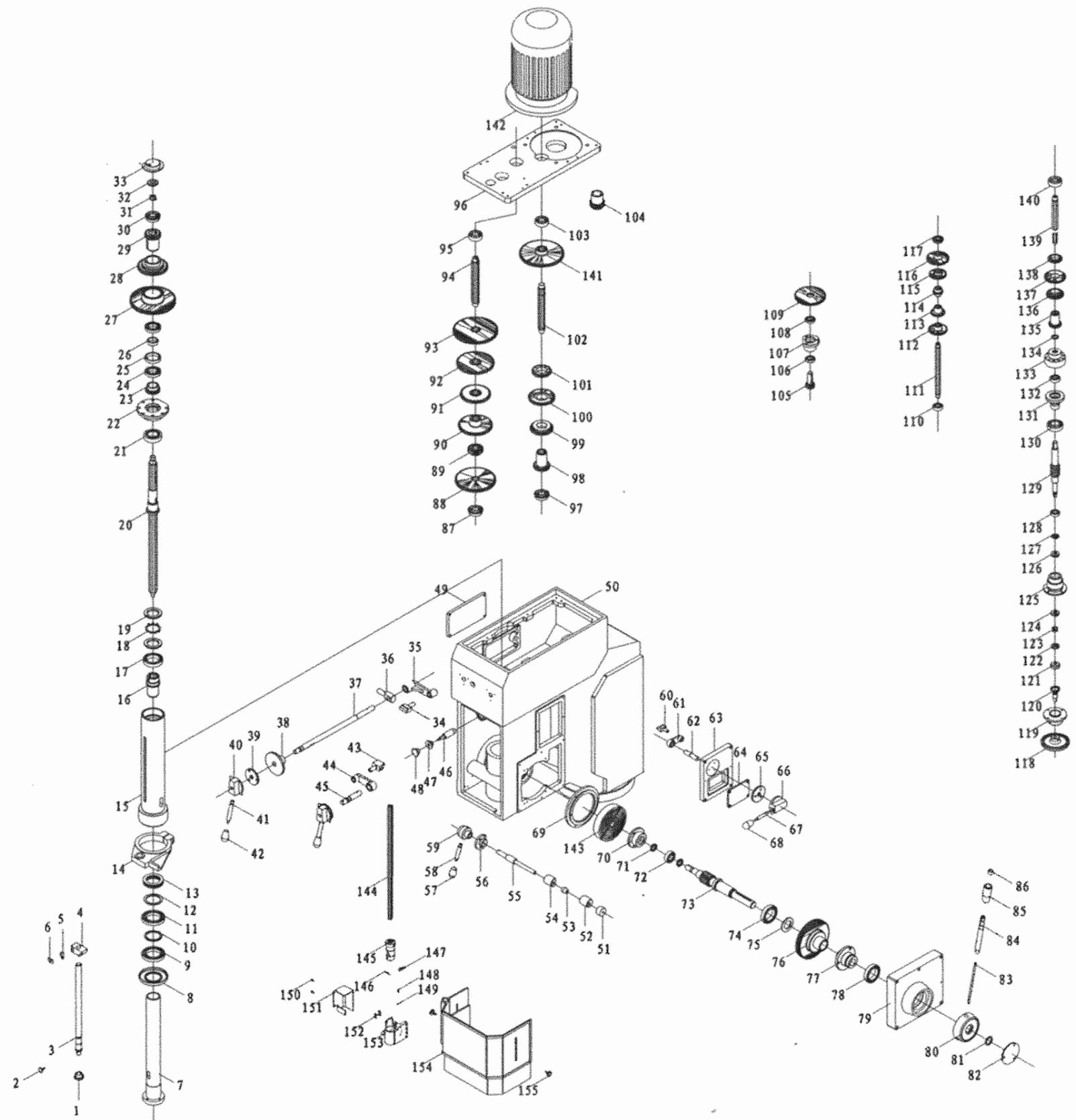
drawing (1) Picture of dimension of spindle box parts structure
